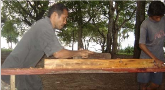
A local skilled in carpentry using a manual plane to shave the timber
